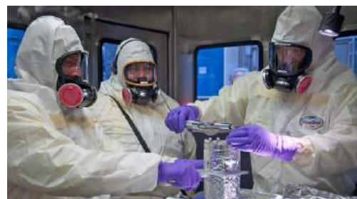
LANL employees working in a downdraft room in the plutonium facility. The airflow in a downdraft room creates a safe environment required to perform certain types of work in pit production.
